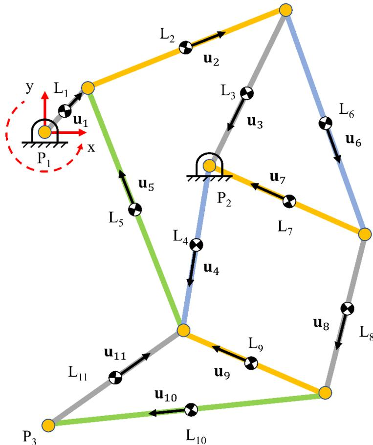
Figure 1: Planar Jansen mechanism discretized with Fully Cartesian Coordinates [1].
