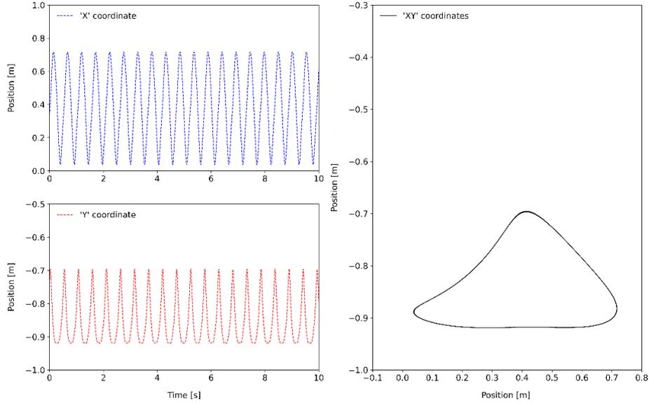
Figure 2 Planar Jansen mechanism:  $x$  and  $y$  coordinates of point  $P_3$ .
