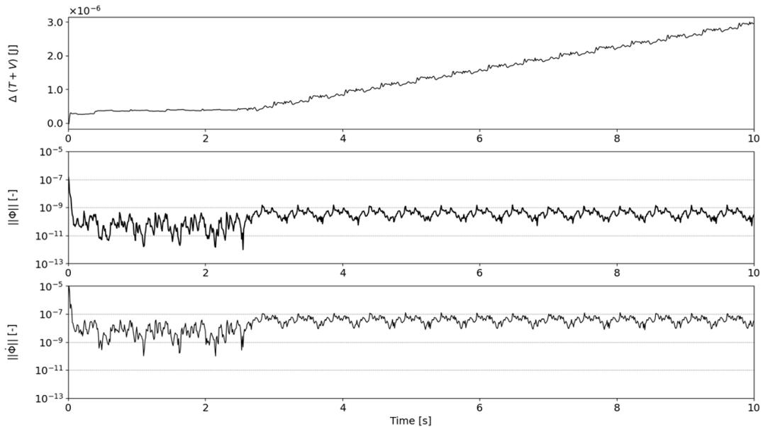
Figure 3: Variation of the mechanical energy of the system and the constraints violations of position and velocity (logarithmic scale).
